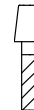
V Add $40 In-Set Pivot For mounting into horizontal surfaces. Requires a hole 0.65" in diameter
